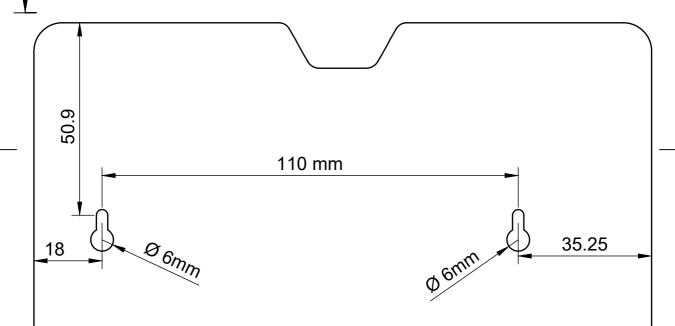
Drilling Jig / Bohrschablone für / for duraSign Pad 4.3 duraSign Pad 4.3 Biometric duraSign Pad 5.0 duraSign Pad 5.0 Biometric
